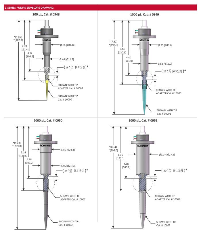
\*Note: Each tip is designed to seal within the reference gap dimension shown. Customers should perform their own testing to determine optimum force/location for sealing and tip stripping.
