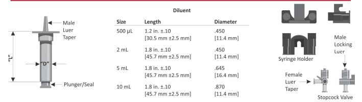
**Diluent Syringe** (For use with pumps with valves) Designed for use with the TriContinent valve, the polycarbonate valve has luer fittings, one male and one female. One fitting is positioned upward and is typically used for liquid output for ease of priming.
