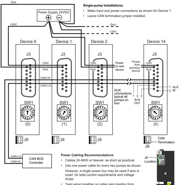
Twist wires together on cable pairs leading from power supply directly to pump.
