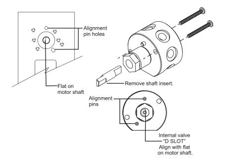
Figure 6-3. 6WD valve interface (C3000MP and C24000MP only)
