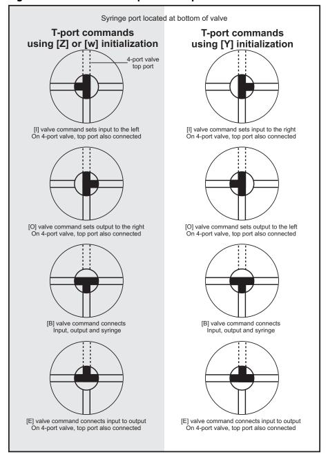
Figure 5-3. Positions for 3-port and 4-port T valves
