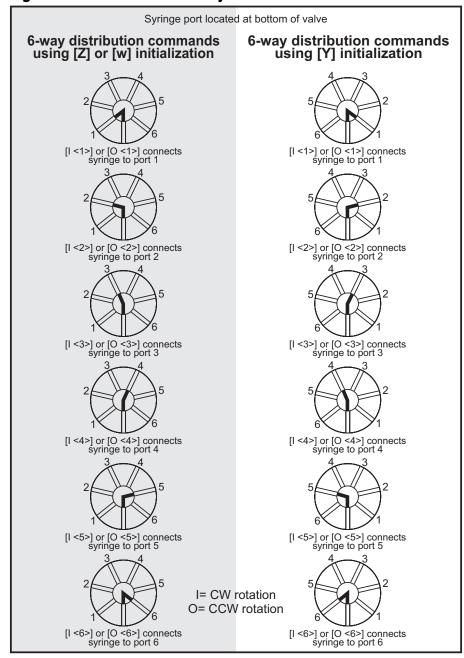
Figure 5-6. Positions for 6-way distribution valve
