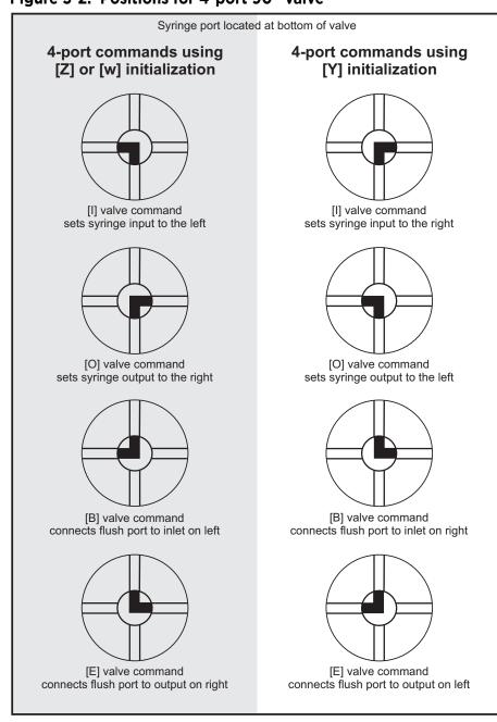
Figure 5-2. Positions for 4-port 90° valve
