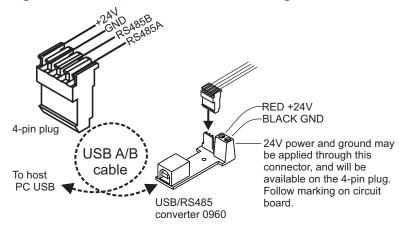
Figure 4-4. USB/RS485 converter wiring detail
