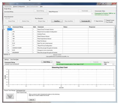
**Streaming Data Chart.** The Streaming Data Chart shows streaming data from an Air-Z pump in real time. The chart shows moving plunger position, pressure count, and optionally capacitive count (Air-Z Premier only). This information assists in determining optimal settings for liquid level operations. Liquid level operations are described in the product manual.
