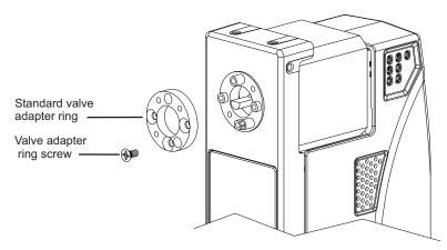
2. Install multi-port adapter ring (7809-37), using two screws supplied with the adapter ring. Keep the countersunk holes to the front (Figure 9-2).
