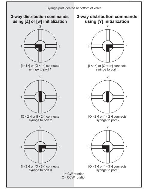
Figure 5-5. Positions for 3-way distribution valve (U11 select)
