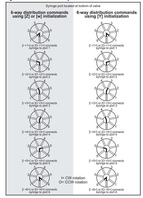
Figure 5-7. Positions for 6-way distribution valve
