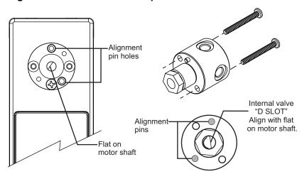
Figure 9-4. Valve installation, 6WD valve
