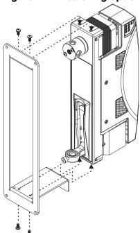
Figure 4-2. Attaching optional adapter panel to pump
