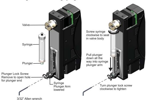
Figure 6-1. Installing syringe
