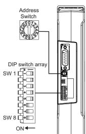
Figure 9-5. DIP and address switch locations.
