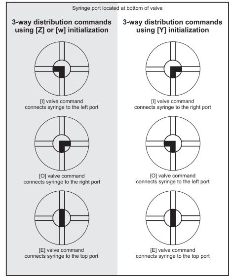
Figure 5-4. Positions for 3-way distribution valve (U4 select)
