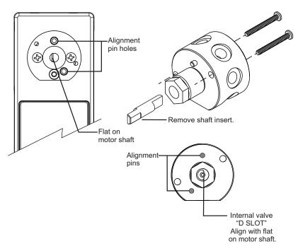
Figure 6-3. 6WD valve interface
