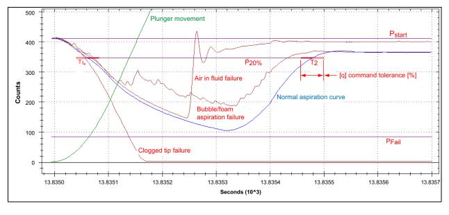
Figure 5-4. Example traces using time intersect
