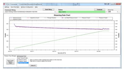
**[q] command tool.** The [q] command tool helps the user determine the operation validation [q] command arguments, <n1> and <n2>. Operation validation monitors fluid operation and detects tip clogs, aspiration of air or bubbles, and failed dispenses. It also verifies that the expected amount of fluid was handled.
