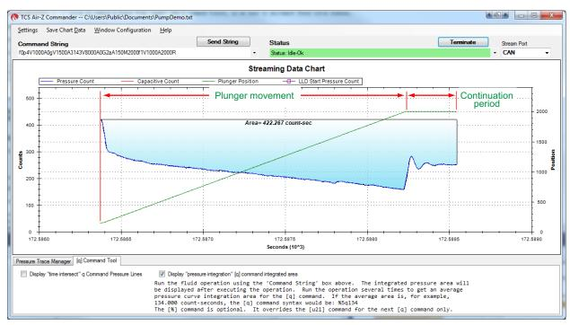
Figure 5-6. Aspiration validation using pressure integration
